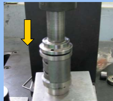
28) CYLINDER, FRONT PALTE, BEARING(629ZZ) 조립
