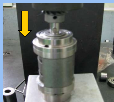
29) SPACER, KEY, DRIVING GEAR 조립
