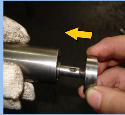
14) SPACER, FRONT PLATE 조립
