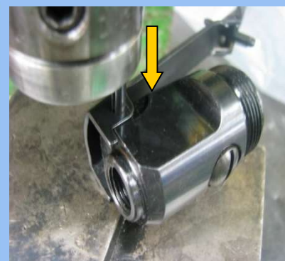
11) HANDLE BODY + SPRING PIN 조립
