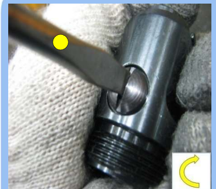
6) VALVE PLUG 조립
