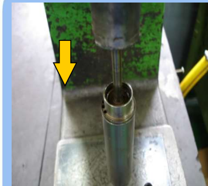
6) ROTOR, REAR PLATE 분해
