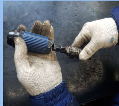
20) CASING + MOTOR ASSY 조립
