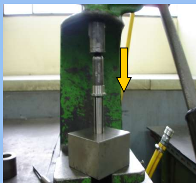
10) REAR PLATE + ROTOR 조립
