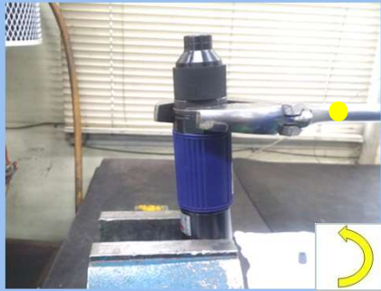
55) CASING에 COLLECT CHUCK CASING 조립-2
