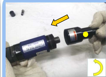
54) CASING에 COLLECT CHUCK CASING 조립-1
