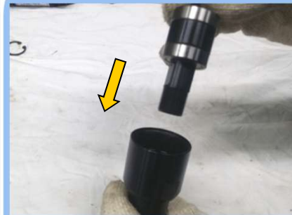
50) COLLECT CHUCK 조립
