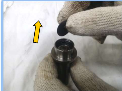
26) REAR PLATE SPACER 분해
