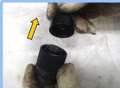
2) AIR INLET BUSHING 분해
