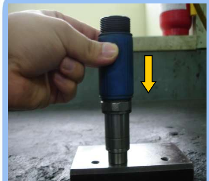
24) OUTER RING, MOTOR ASSY + CASING 조립
