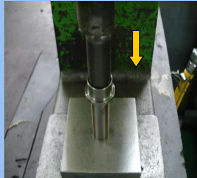
17) ROTOR + REAR PLATE 조립
