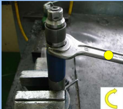
4) WHEEL SPINDLE CASING 분해
