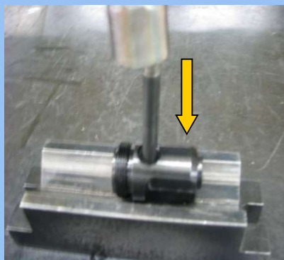
4) STEEL BALL 조립 (BALL PRESSING)
